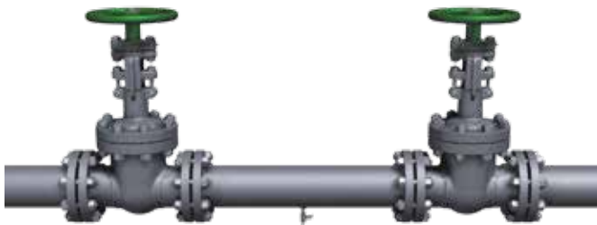
The double block-and-bleed system (as shown above) required the use of two valves and a spool piece. A bleed valve was used to drain the spool and verify seal integrity.
